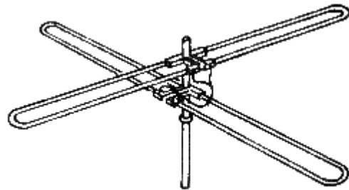
In practice it may not be possible to have the driven element of a crossed yagi exactly in line. A centimetre or two apart on the same boom is Ok. The circular polarisation is achieved by feeding power to one antenna and using a 90 degree (quarter wave) delay line between the feed points to get power to the second yagi.
